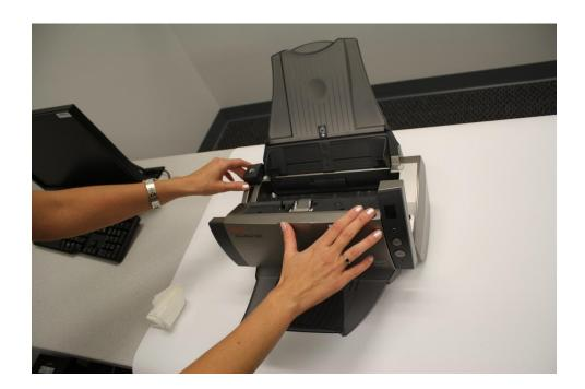
• Dampen a soft cloth with some Isopropyl rubbing alcohol (95%). Wipe the feed roller from side to side. Rotate the roller to clean its entire surface.
