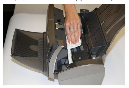
• When you have finished cleaning the scanner, close the scanner cover. Power the scanner on.
